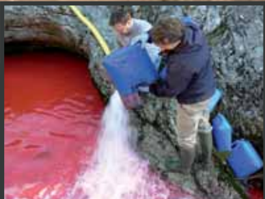
Injecting a tracer to monitor groundwater flow to characterize karst systems.
